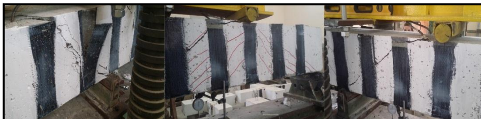
Figure (14): Debonding of CFRP for Beam Specimen (SCC-R0-90°)
