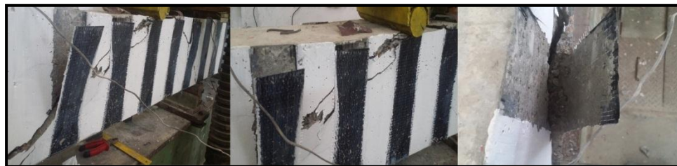
Figure (15): Debonding of CFRP for Beam Specimen (SCC-R3-90°)
