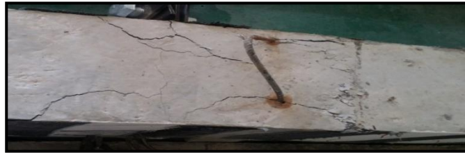
Figure (13) Cracks on the Top Surface of Beam Specimens
