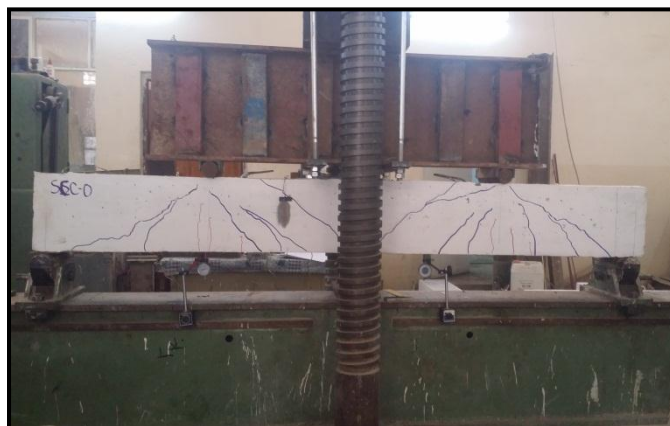
Figure (10) Beam Specimen Setup
