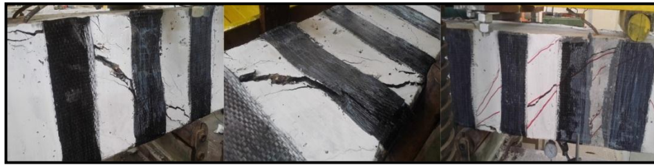
Figure (16): CFRP Rupture for Beam Specimen (SCC-R5-90°)
