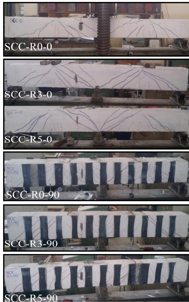
Figure (11) Crack Pattern
